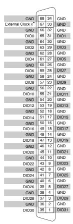
\* x is the connector number. External Clock x is an input only.
